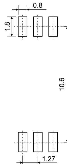
Fig. 15.2 Lead forming and taping option (LF4), (TP4)
