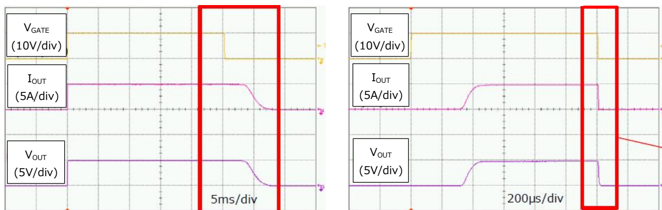
Fig 3.5 Differences in waveform with or without auto-discharge function (TCK401G)
