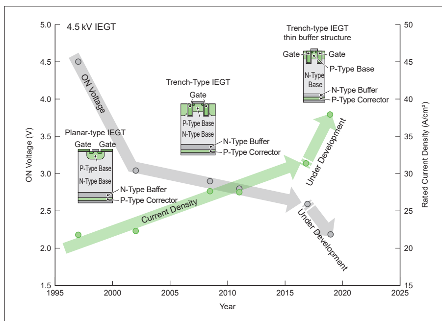
(Figure 6) : Trends in performance of high-voltage injection enhanced gate transistors (IEGTs)
