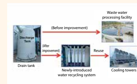
A recycling system was introduced to treat the water used in the process after draining and being reuse in the cooling tower
